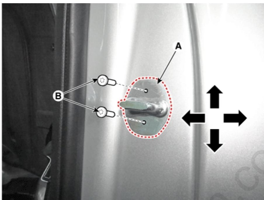
3. Tap on the striker with a plastic hammer to adjust the striker. The striker will not move much, but will give some adjustment.
