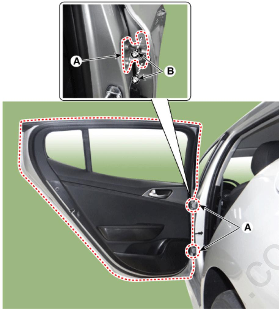
4. Grease the pivot portions of the hinges indicated by the arrows.
