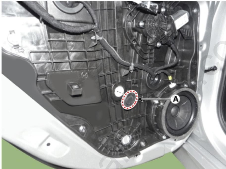
3. Carefully move the front door window glass (A) until the glass mounting bolts are visible, then loosen them.
